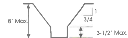
Figure 3. Type A Soil Unsupported, Vertically Sided Lower Portion, Maximum 8 Feet in Depth
